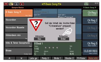
The installation data is now available on the stick and can be installed as described below. **But first a tip**: Please, delete the archive file again from your factory data stick after installing the data. Otherwise, the display will always ask whether the file should be unpacked when you insert the stick into the organ, since archive files are automatically recognized. The unpacking has now already taken place and the archive file can thus be deleted from the stick, it is no longer needed.
